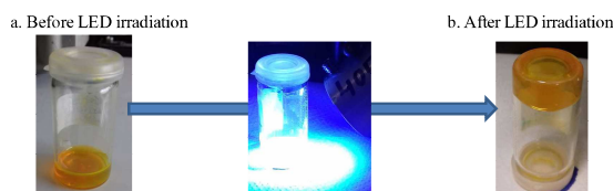
Figure 2: Hydrogel formation: polymerization of HEMA in water under LED@405 nm with NHC-Borane PIS.
